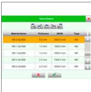
Automatic material sheet thickness adjustment, controlled by ProLink X
